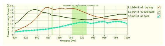
Sensitivity&Read Range Test power: 4W EIRP
